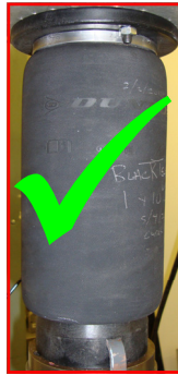
Figure (e). Three air spring views: inflating correctly (✓), buckled and uninflated (X), and buckled and inflating incorrectly (X)
